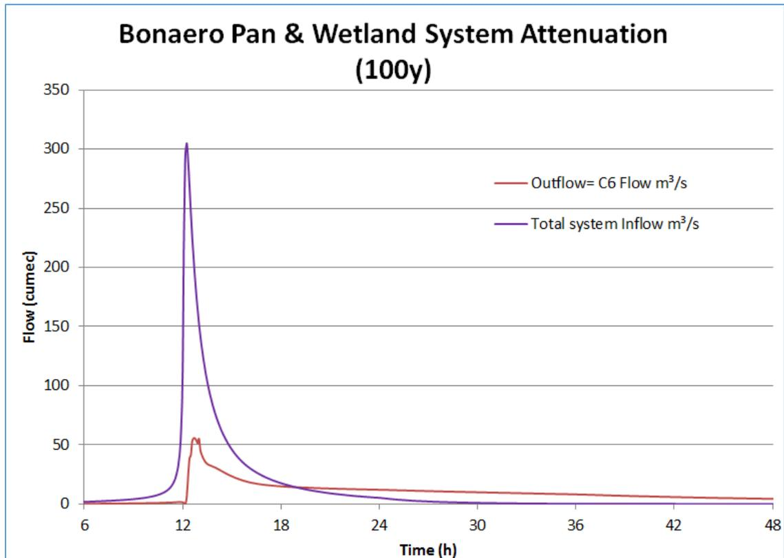
Figure 48: Attenuation effect of the entire Bonaero pan and wetland system on the estimated 100 year flood event (PCSWMM simulation)
