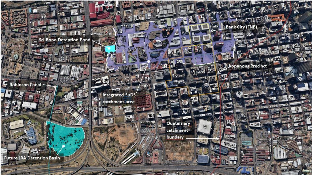
Figure 20: The CBD sub-catchment (blue shaded ground surface) used to analyse an integrated SuDS treatment train.
