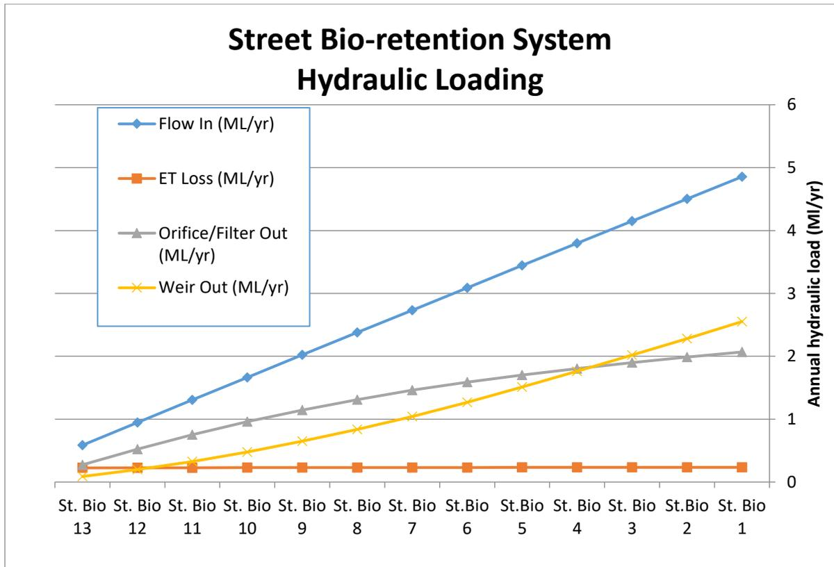
Figure 30: Increasing hydraulic loading along Street Bio-retention treatment train
