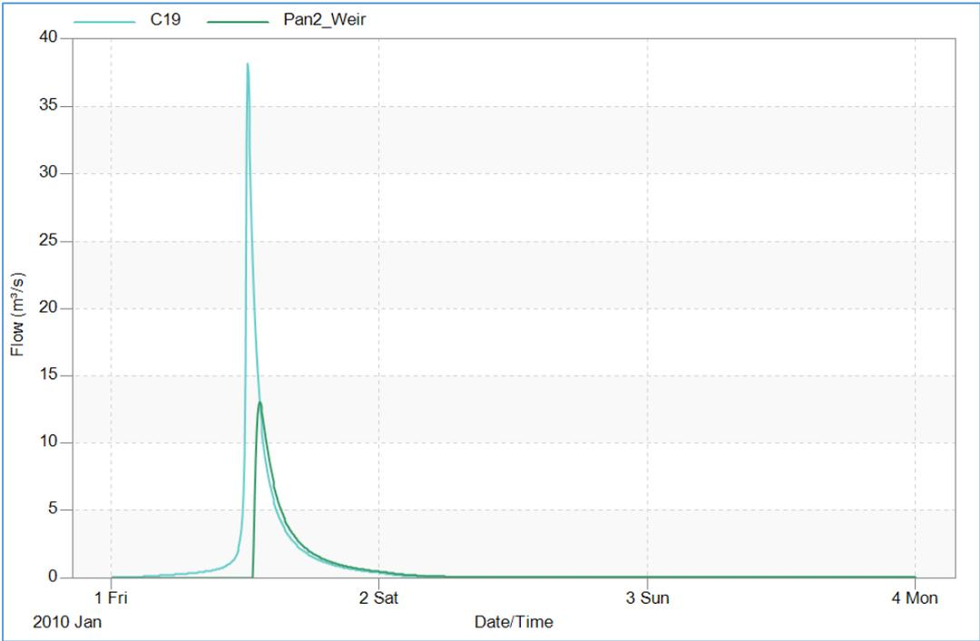
Figure 46: Pan2 - attenuation of the estimated 100 year flood hydrograph (PCSWMM simulation).
