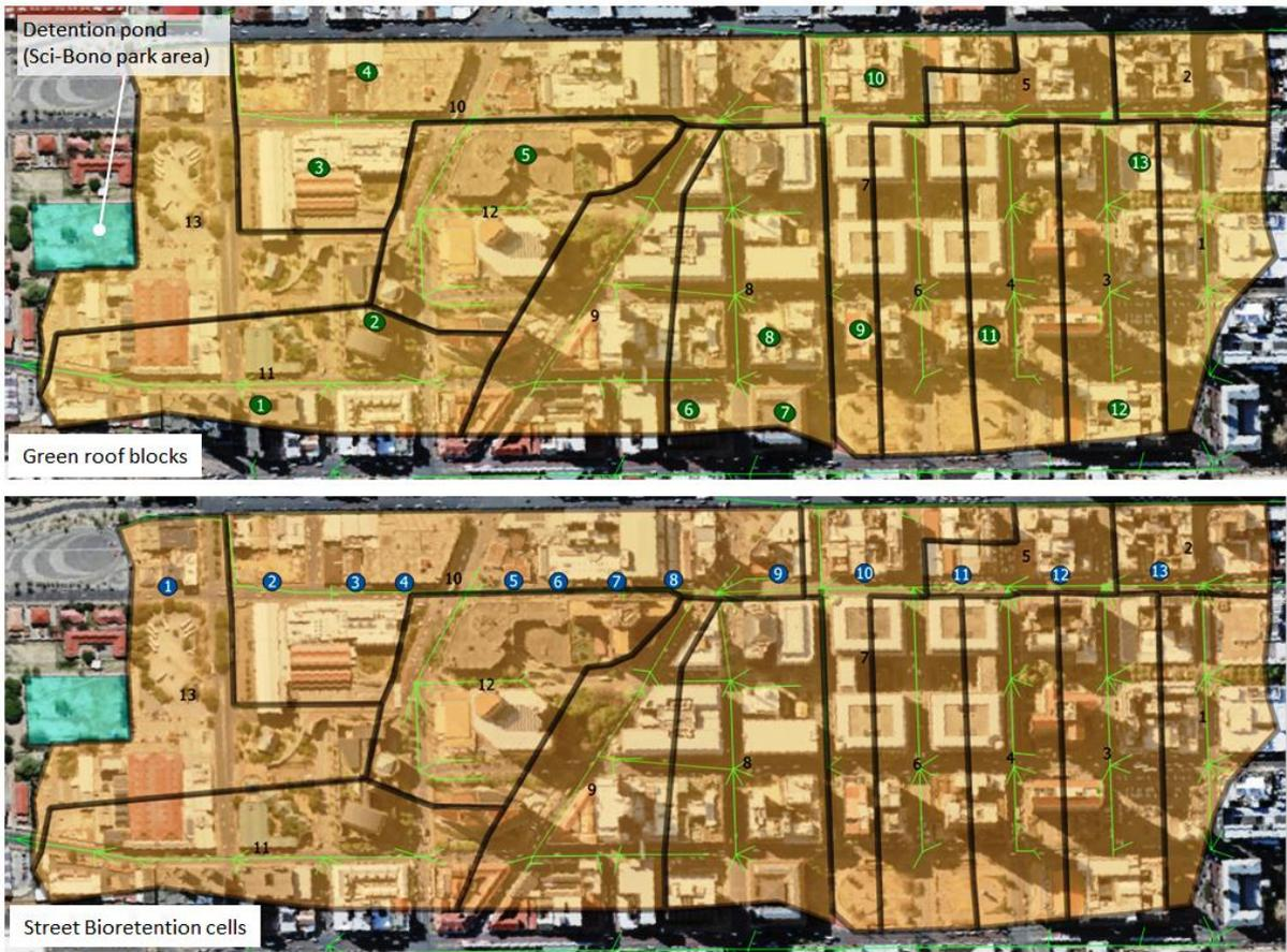
Figure 21: CBD Sub-catchment integrated treatment train incorporating green roof (top) and street level (bottom) interventions, and a detention pond in the Sci-Bono park area.
