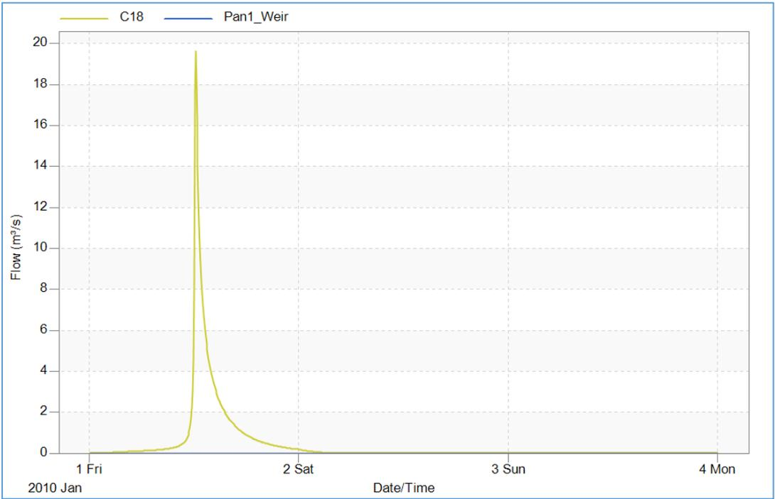
Figure 45: Pan1 - attenuation of the estimated 100 year flood hydrograph (PCSWMM simulation). See further explanation in figure above; outflow zero.
