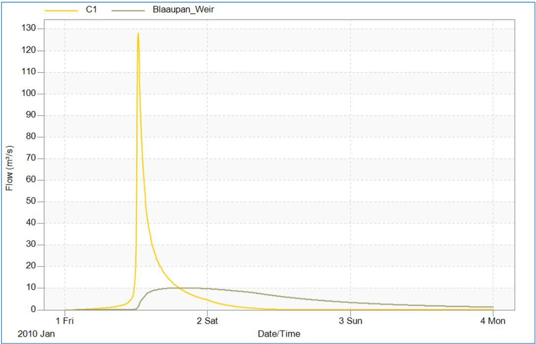
Figure 44: Blaauwan – attenuation of the estimated 100 year flood hydrograph (PCSWMM simulation using design flood; dates are not actual dates), with C1 being the inflow hydrograph and the weir being the outflow hydrograph
