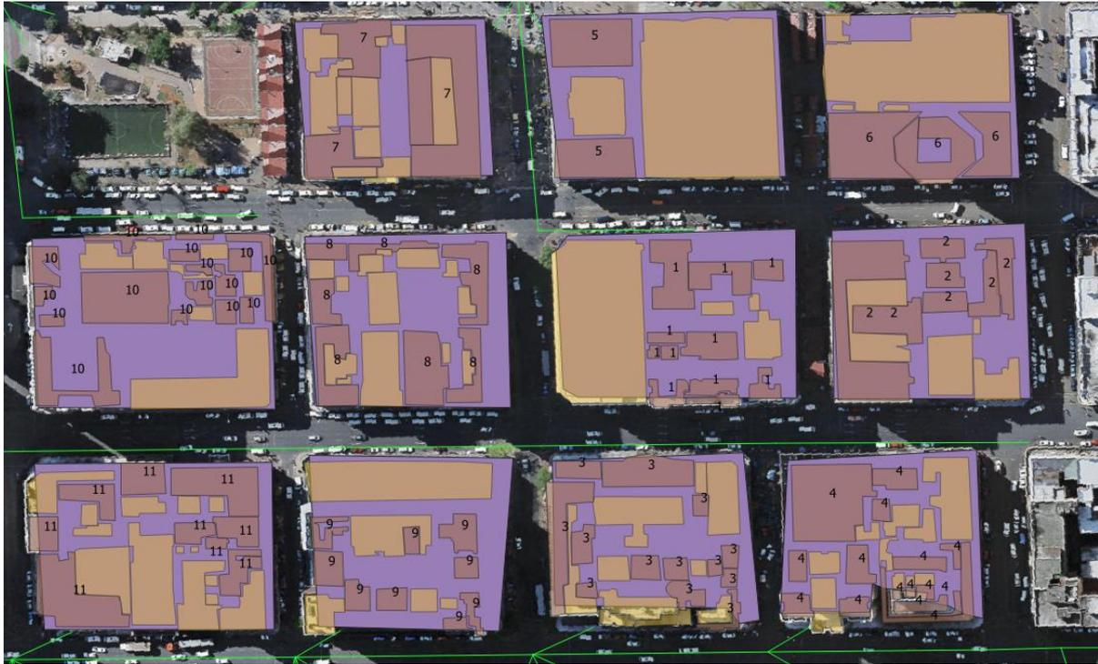
Figure 11: CBD roof space - Analysis of flat roof areas (numbered polygons) per block in the CBD study area.
