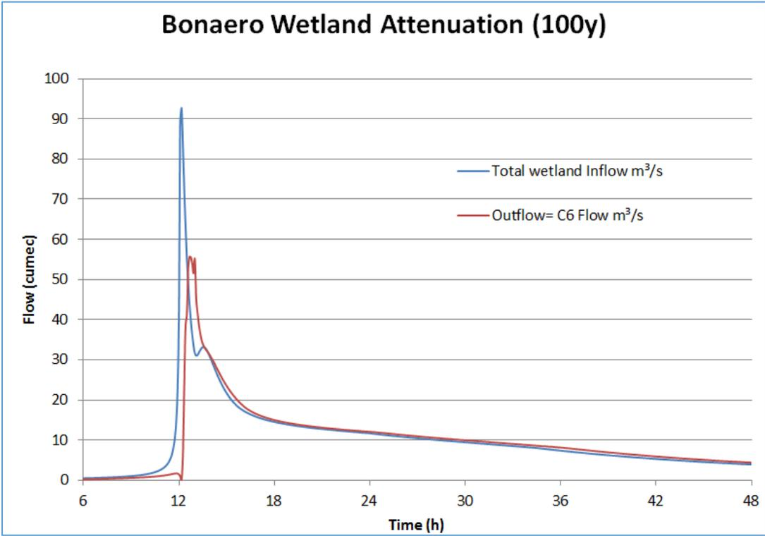
Figure 47: Attenuation effect of the Bonaero wetland on the estimated 100 year flood event (PCSWMM simulation)
