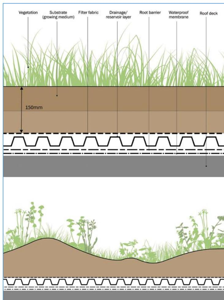
*Figure 18: Extensive green roof concept (top) and example for enhanced biodiversity potential (bottom). (after Woods-Ballard, et al, 2015). [NB copyright]*
