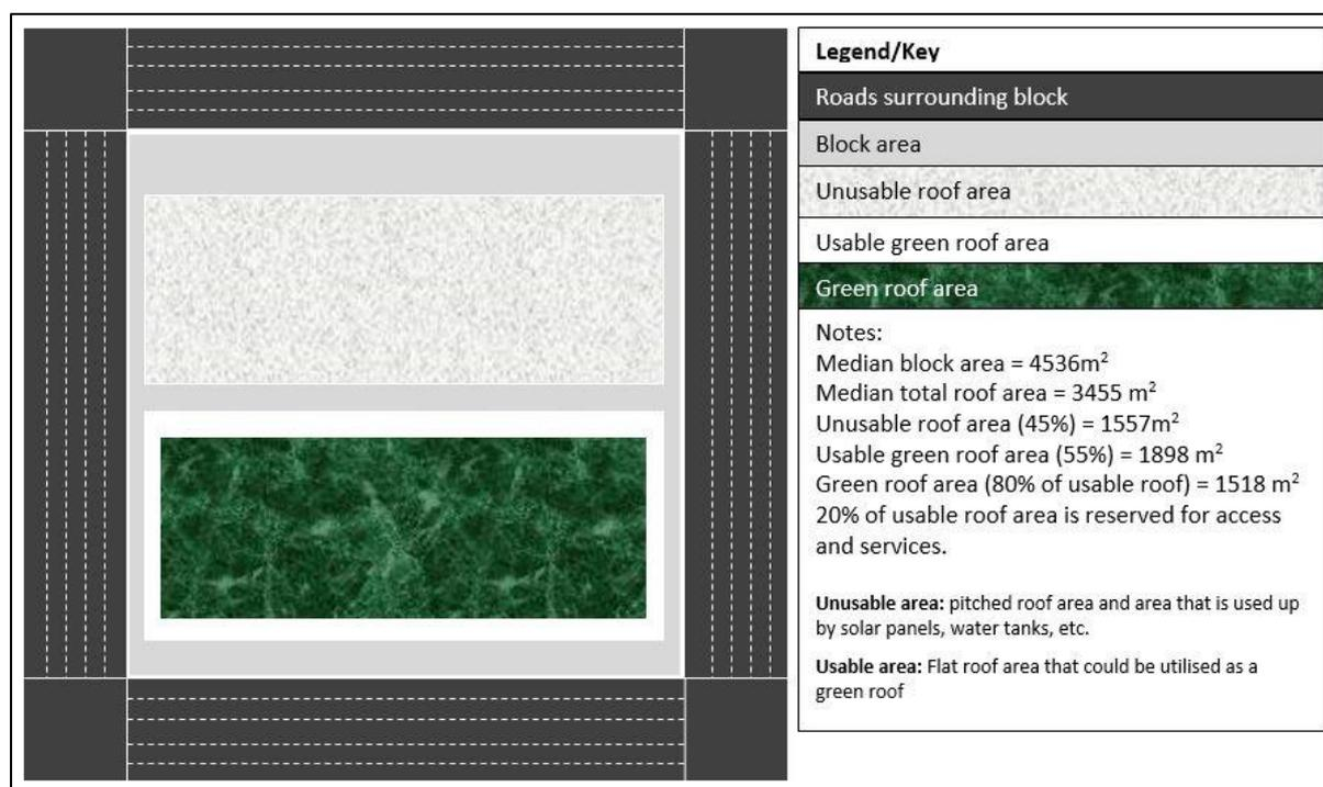
Figure 17: Schematic representation of the median roof areas for the green roof analysis.
