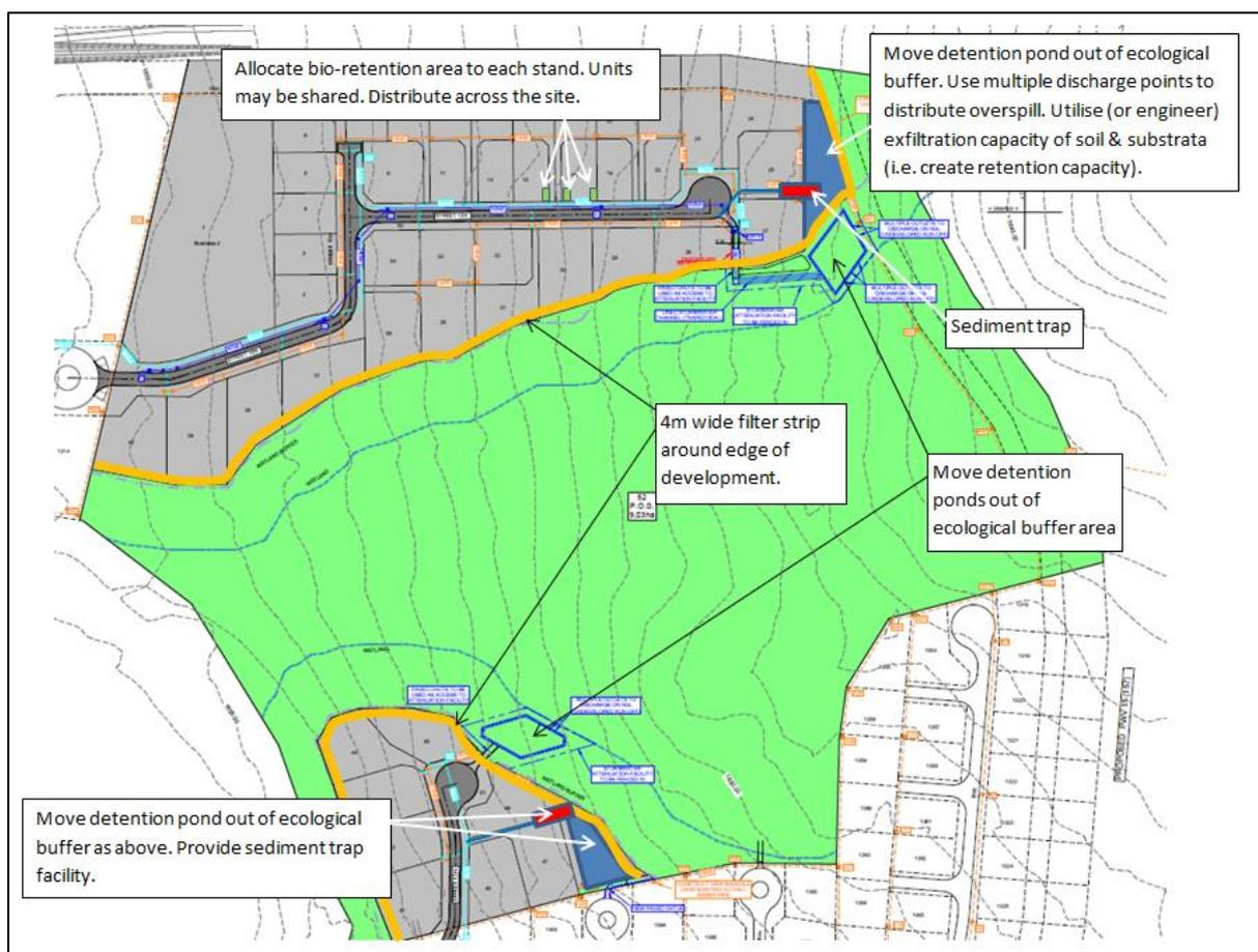
**Figure 58:** SuDS concept for Erf1317 (adapted from Protech, 2016)
