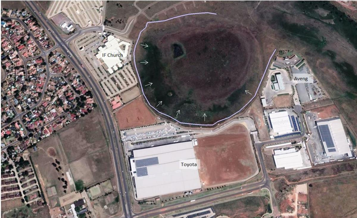
Figure 53: Pan 1 showing the estimated location of the bioswale and expected points of stormwater discharge.
