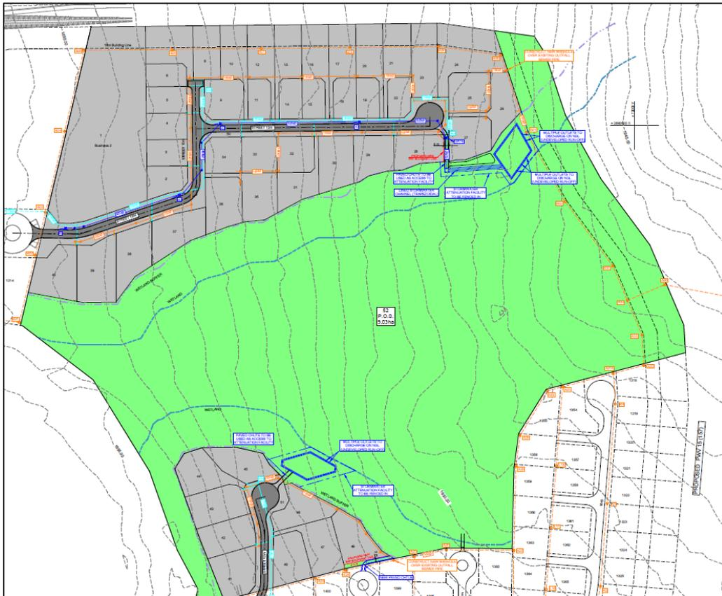
**Figure 57: Development plan for Erf 1317 showing delineated wetland and proposed attenuation ponds in wetland buffer area (Protech, 2016)**
