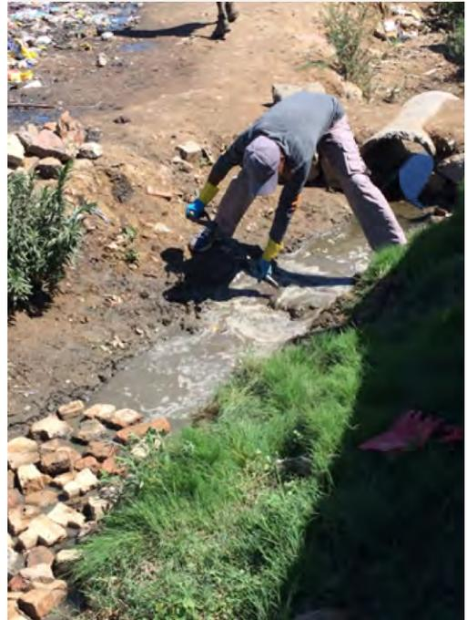
*A reduction in water runoff was observed in both channels, indicating the success of the semi-pervious channel in improving the water management at this small scale*
